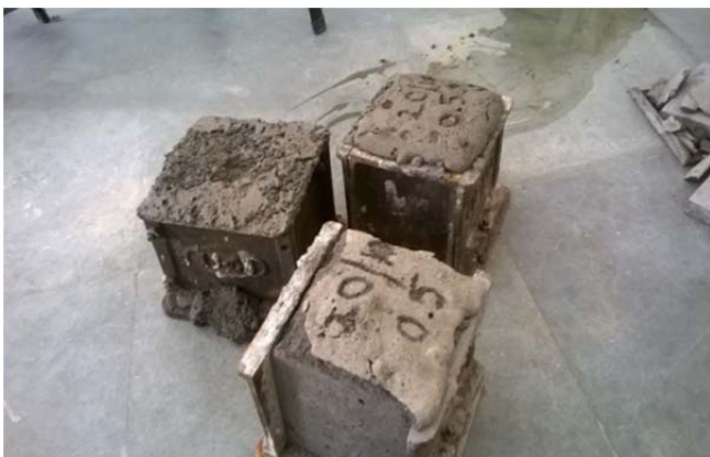
Fig. 12: Effect of Aluminum powder (effervescence)
