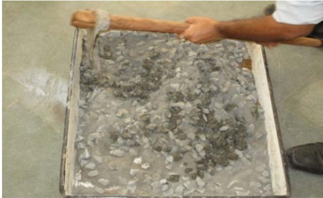
Fig. 10: Preparation of concrete mix
