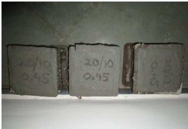
Fig. 11: Removal from cube mold and ready for curing
